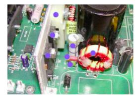
The SiC diode has very low reverse current so can be used without additional components, resulting in space saving on the board (as shown in Figure 2), lower assembly costs and greater reliability. In addition, because almost no power is lost due to reverse current, the efficiency of the power supply is increased by around 1% - a significant improvement.
