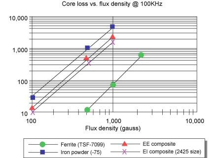
Developments in composite magnetic materials will have significant impact on power supply design over the next few years, their take-up being limited only by availability and price. As with most new technologies, availability of composite cores is restricted at present to relatively few suppliers.
